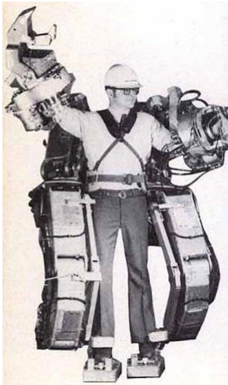
Figure 2: General Electric's exoskeleton, the „Hardiman” [4]
