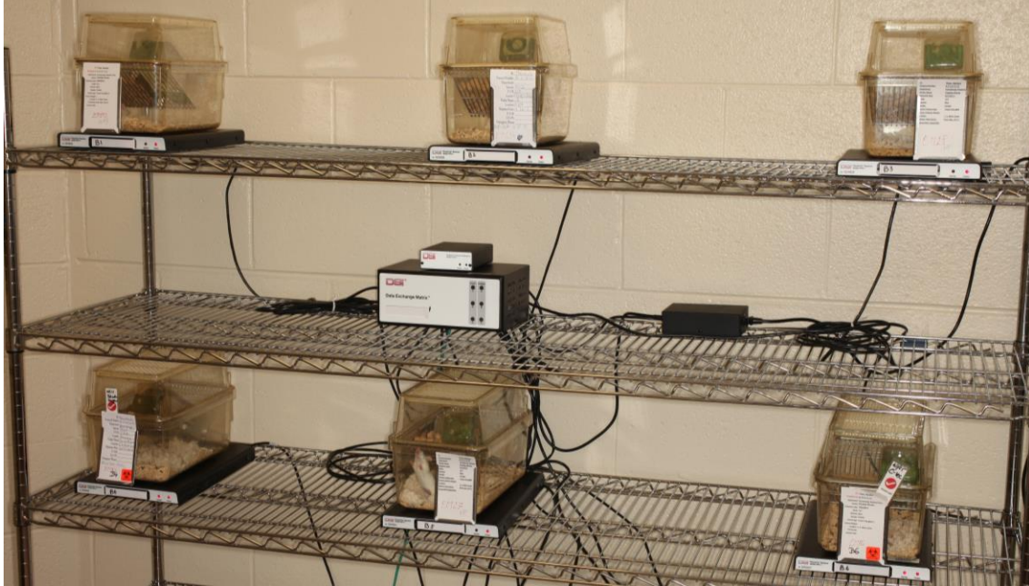
Figure 6. Telemetric blood pressure monitoring system. Mice were kept separately in standard-size filter top rodent cages. Blood pressure monitoring was started three days after the catheter implantations on conscious, unrestrained animals, and was continued until postpartum day (PPD) 7 using the Dataquest A.R.T. 4.31 acquisition and analysis system (Data Sciences International). Freely moving mice housed in plastic cages were placed on the top of the receiver, and the implanted telemetric devices transmitted the data to the receiver with radio frequency. The photo is courtesy of the Perinatology Research Branch, NICHD, NIH, DHHS.
