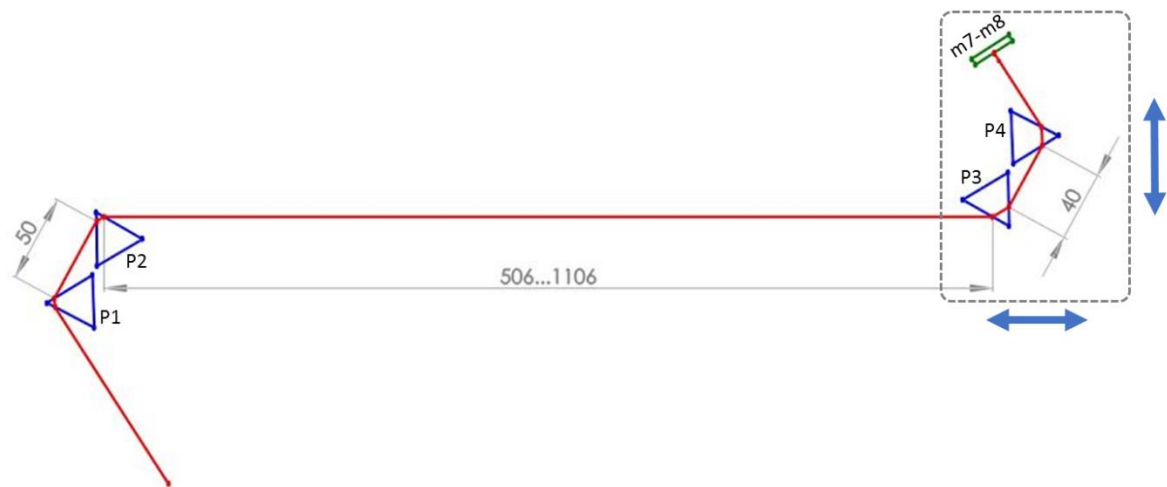
Figure 18. Four-prism compressor unit. Mechanical model for realization of the compressor with the arm lengths designed by my calculations. P1-P4: prisms; m7-m8: broadband dielectric mirrors; gray numbers: distances in mm; blue arrows: direction of movement of the motorized mirrors. See details in the main text.)
