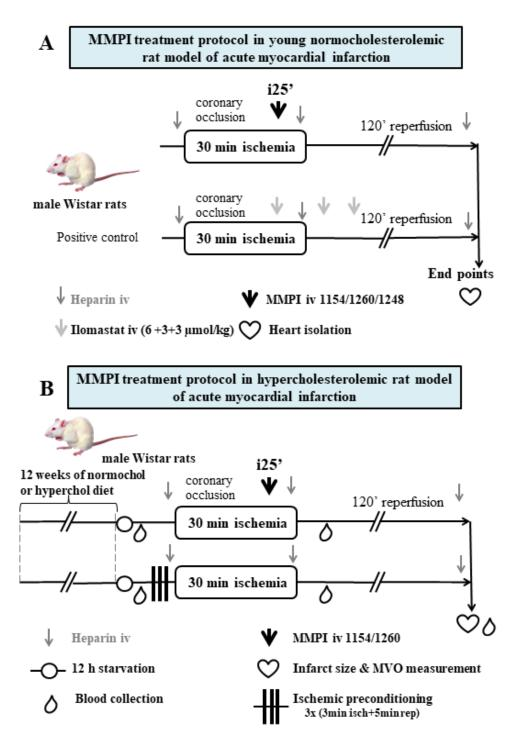
**Figure 12.** Experimental protocol of *in vivo* acute myocardial infarction in A) normocholesterolemic and B) hypercholesterolemic and age-matched normocholesterolemic rat model. MMPI: matrix metalloproteinase inhibitor, iv: intravenous, MVO: microvascular obstruction.
