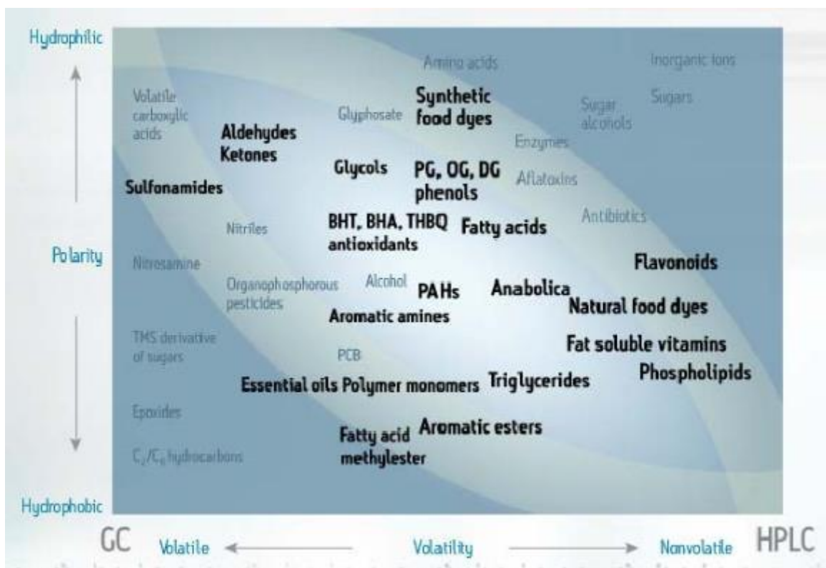
Figure 13. Potential applicability of supercritical fluid chromatography (compounds which can be analyzed by SFC are marked black) (www.waters.com,2012)
