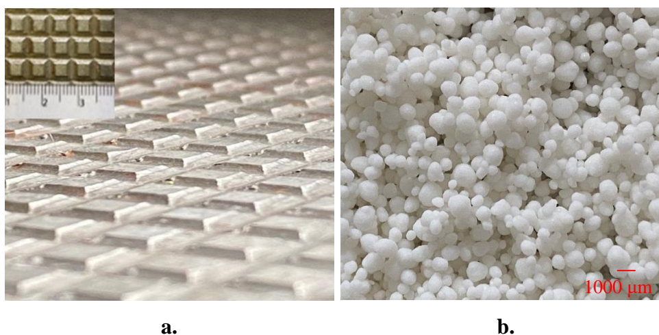
Figure 14. a.) Spheroniser disc surface b.) wet spheronised micropellet particles
