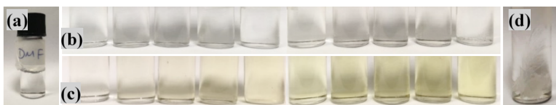
Figure 4.12 a) DMF b) LiBr 1-10w/w% c) KI 1-10w/w% d) 10w/w% LiCl 10w/w% crystal growth [24]
