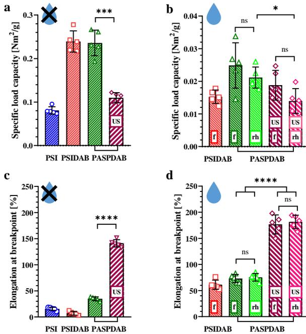
Figure 41 Specific load capacity (a, b) and elongation at breakpoint values (c, d) of dry (a, c) and wet (b, d) samples measured by a tensile test. The presented data show the average of 5 independent measurements. The error bars correspond to the standard deviation of the mean. The "\*" indicates statistical significance exists between two groups (one-way ANOVA, \* $p < 0.05$ ; \*\* $p < 0.01$ ; \*\*\*\* $p < 0.0001$ ).
