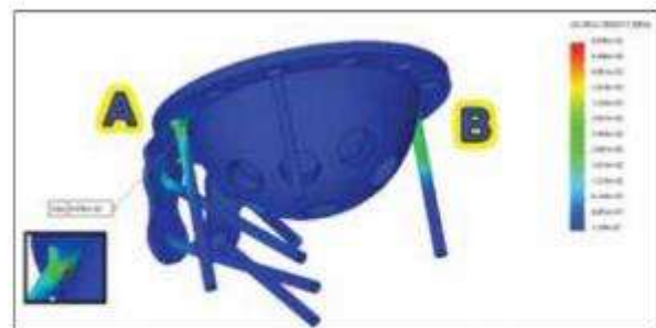
Figure 4. Implant strain during weight-bearing (main load-bearing screws noted with 'A' and 'B').
