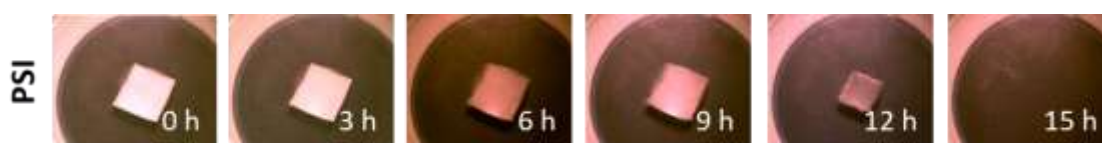
Figure 49 Hydrolysis of electrospun PSI fiber membrane in pH 8 buffer solution
