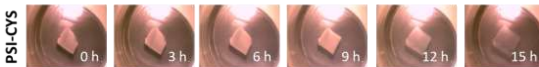
Figure 50 PSI-CYS fibrous membrane in pH 8 buffer solution during hydrolysis
