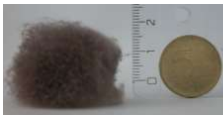
Figure 34 3D structure of magnetite loaded PSI fibers
