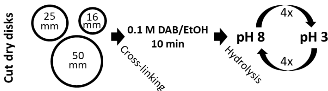
Figure 23 Schematic of pH responsivity test of PASP-DAB
