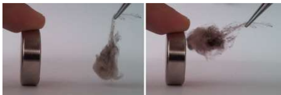
Figure 42 Attraction of electrospun fiber membrane loaded with magnetic particles by non-uniform magnetic field.
