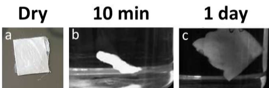
Figure 43 Dry PSIsp10 sample before cross-linking (a); PSI-DAB samples in DMF prepared from PSIsp10 with cross-linking times 10 minutes (b) and 1 day (c)
